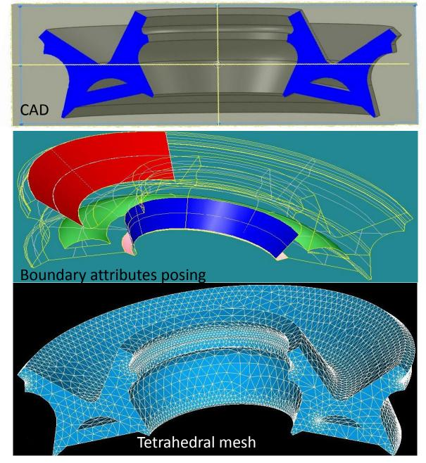
Initial tetrahedral mesh before refinement is shown. The resulting mesh includes 10<sup>8</sup> cells and more.
