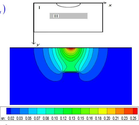
1.5·10<sup>9</sup> mesh nodes K-100 - 100TFLOPs **Contaminant saturation field**
