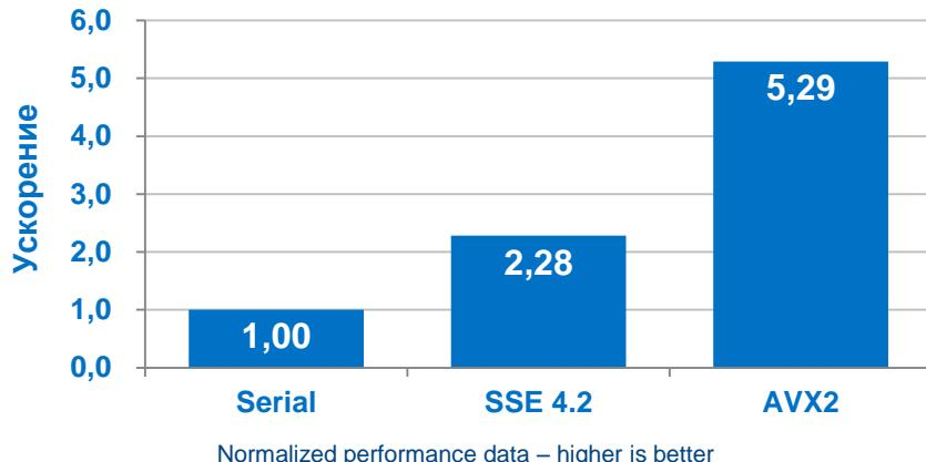
Configuration: Intel® Xeon® CPU E3-1270 v3 @ 3.50 GHz system (4 cores with Hyper-Threading On), running at 3.50GHz, with 32.0GB RAM, L1 Cache 256KB, L2 Cache 1.0MB, L3 Cache 8.0MB, 64-bit Windows® Server 2012 R2 Datacenter. Compiler options: SSE4.2: -O3 -Qipo -QxSSE4.2 or AVX2: -O3 -Qipo -QxCORE-AVX2.
